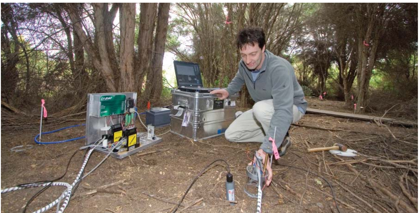
Figure 1: Chamber system used to collect respired air from the soil surface for isotopic analysis
