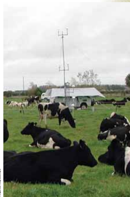
Just part of the scenery: The measuring system for methane emissions, parked in a Canterbury paddock.
