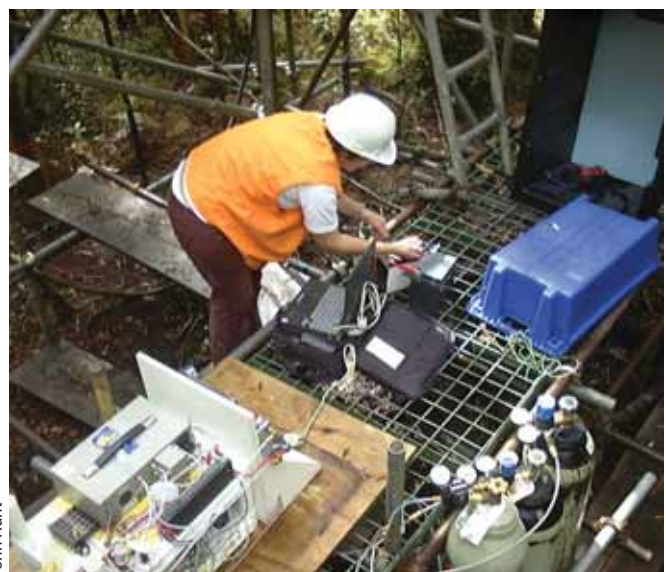
Margaret Barbour preparing instrumentation for measuring water use by mature trees.
