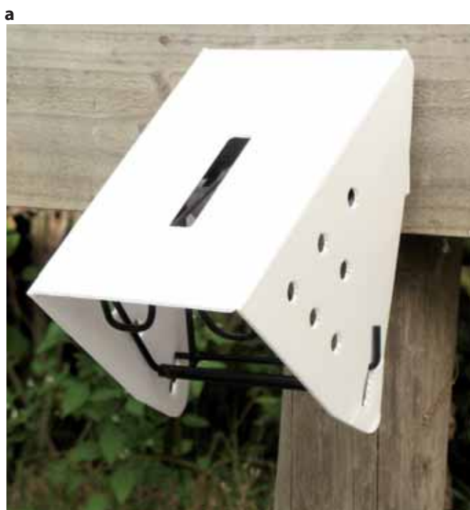
Sentinel possum kill trap equipped with (a) the standard commercial trap cover and (b) a cover fitted with a weka excluder
