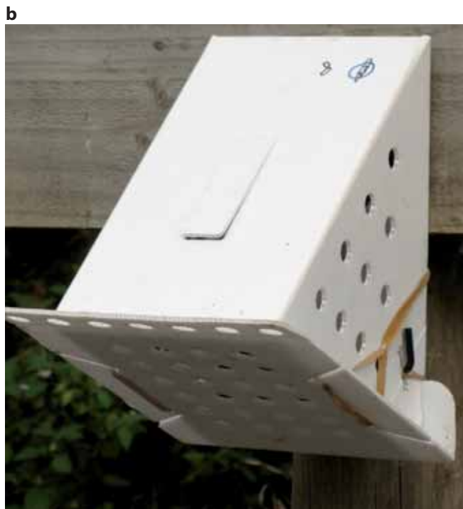
Sentinel possum kill trap equipped with (a) the standard commercial trap cover and (b) a cover fitted with a weka excluder
