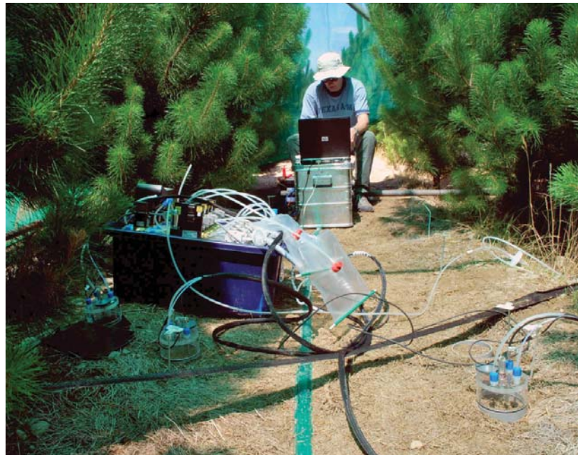
FIGURE 1 Equipment used to collect the soil surface CO 2 efflux in order to measure its isotopic composition.
