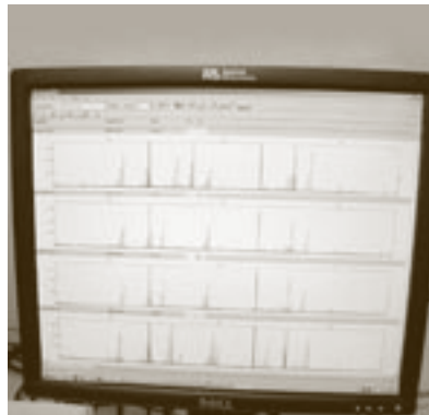
After analysis, unique DNA profiles from different possums can be identified. In the figure, the middle two rows represent samples from the same possum.
