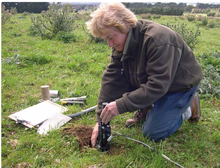
■ Carolyn Hedley testing a smart sensor to measure reflected light energy from soil.
