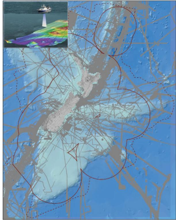
**FIGURE 4** Map of the New Zealand Exclusive Economic Zone and Extended Continental Shelf showing the extent of swath mapping coverage. Inset is a cartoon of swath mapping being carried out by the R.V. *Tangaroa*. The swath width is up to seven times the depth of water below the survey vessel, thus swath mapping in deep water is generally faster and less expensive than mapping the same area of seafloor in shallow water.
