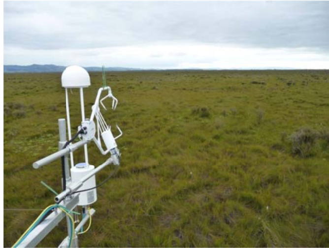
Eddy covariance sensors tower over the Empodisma bog canopy. Photo: D Campbell
