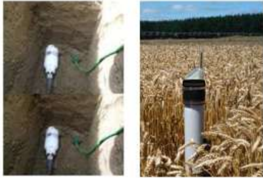
(1) Wireless in-field nodes with sensors attached
