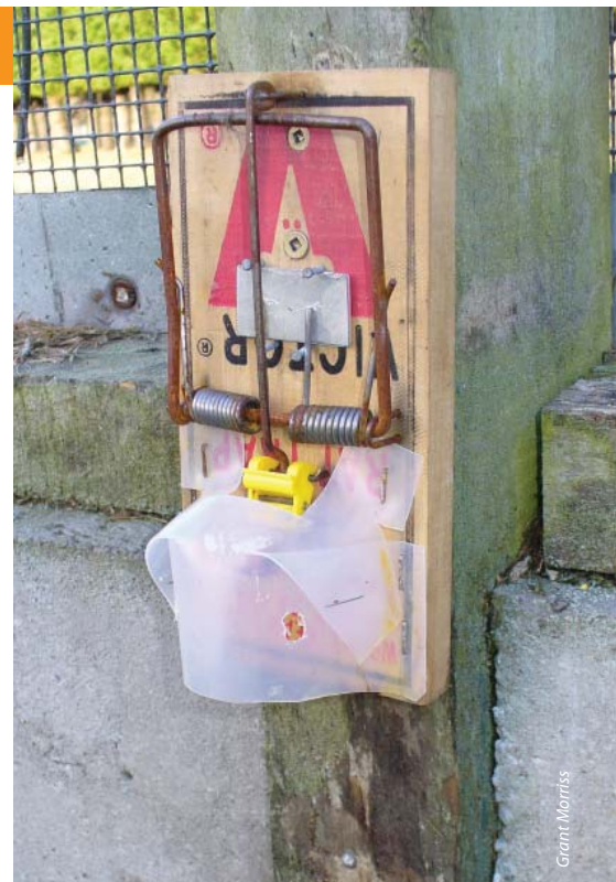
Fig. 1 The Victor® Easy Set® trap set vertically with a shroud to ensure the targeted animal is positioned correctly for a humane kill and that non-target animals are excluded.
