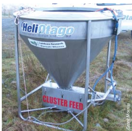
Fig. 3 The Tracmap GPS-controlled Landcare Research/HeliOtago cluster-sowing bucket.
