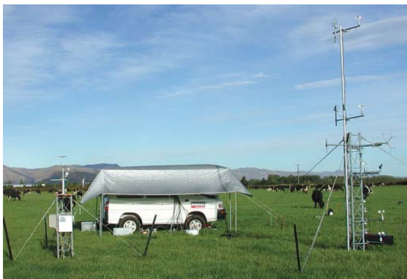
Measuring net methane emissions from grazing dairy cattle and oxidation by soils at the paddock scale, using air sampling lines, micrometeorology and a mobile field laboratory
