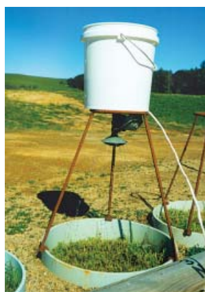
Buried lysimeters with the individual effluent spray applicators
