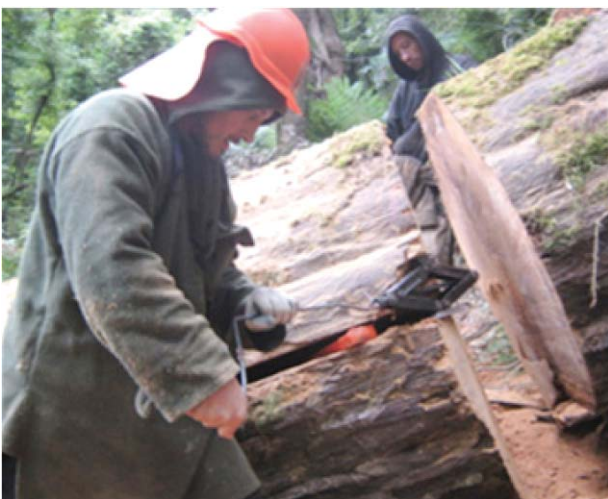
Puke Timoti, resourceful as our logging team is, uses a car jack to split open a huge log.
