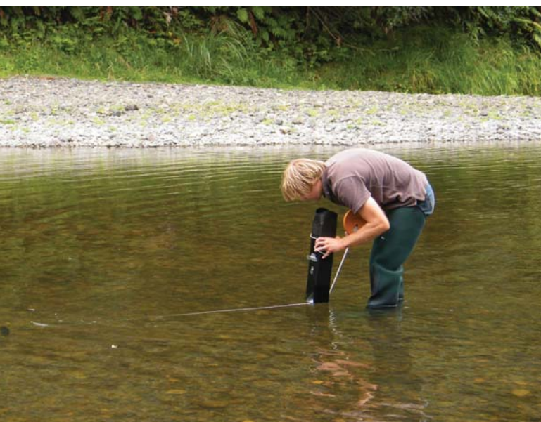
FIGURE 1 Measuring visual water clarity at a river site in the NRWQN. The technician is using an underwater periscope (black item in his left hand) fitted with a 45 degree mirror to view horizontally under the water surface. Visual clarity is the distance (measured by tape measure) at which the visual target (black disc on the left of the image) disappears. The black disc is fixed to a steel pole driven into the river gravel.
