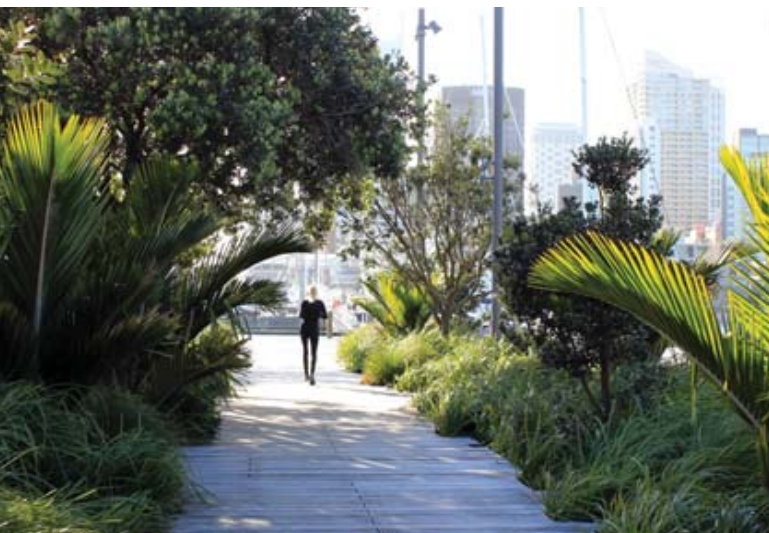
FIGURE 1 Rain gardens at Karanga Plaza, Auckland City intercept, retain and cleanse runoff from adjacent paved surfaces before discharge to the harbour. The rain gardens are functional landscaping using local plants.
