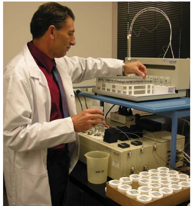
FIGURE 2 Measuring nitrogen and phosphorus in river water samples from the NRWQN on the Flow Injection Analyser (FIA) in NIWA Hamilton's water quality laboratory.
