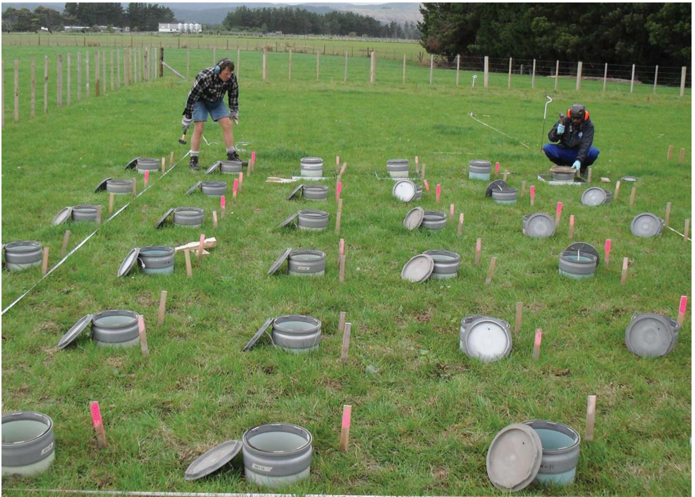
FIGURE 2 Static chambers are installed for field measurements of nitrous oxide emissions from plots treated with and without cattle urine, by Peter Berben (left) and Thilak Palmada.
