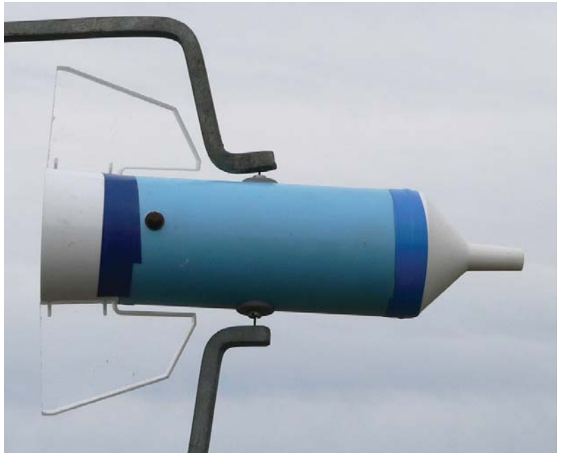
FIGURE 1 Side view of an ammonia sampler, affectionately called “space shuttle”. The sampler rotates itself into the wind (here blowing from right to left). Inside is an elaborate array of metal surfaces coated with oxalic acid that traps the ammonia.
