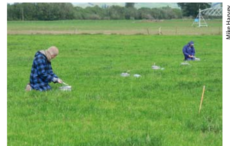
'Bottom up' measurements: Tony Bromley (NIWA) and Jagrati Singh (Landcare Research) help to collect gas samples from chambers.
