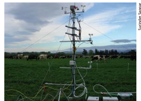
'Top down' measurements: air is sucked from two heights at high velocity and piped to a laser detector.
