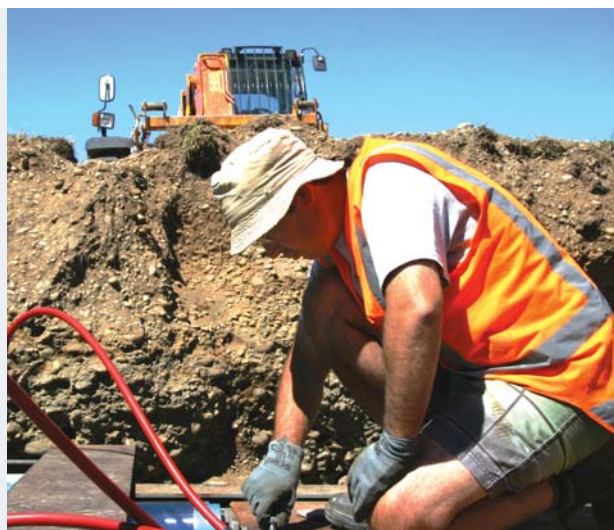
Sam Carrick setting up a large scale lysimeter in stony soil (Caroline King)
