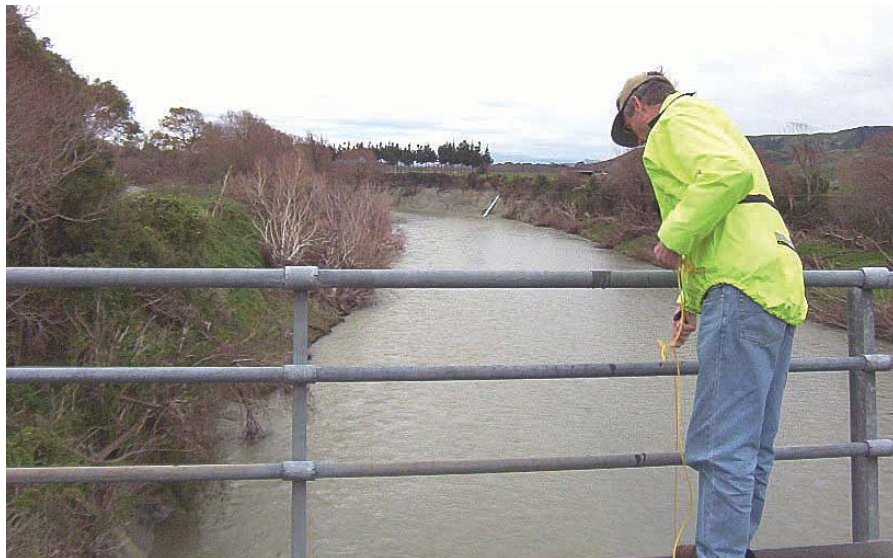
■ Dr Roger Parfitt at the Manawatu River at Hopelands, pulling up a bottle of river water to be analysed for nitrogen and phosphate.
