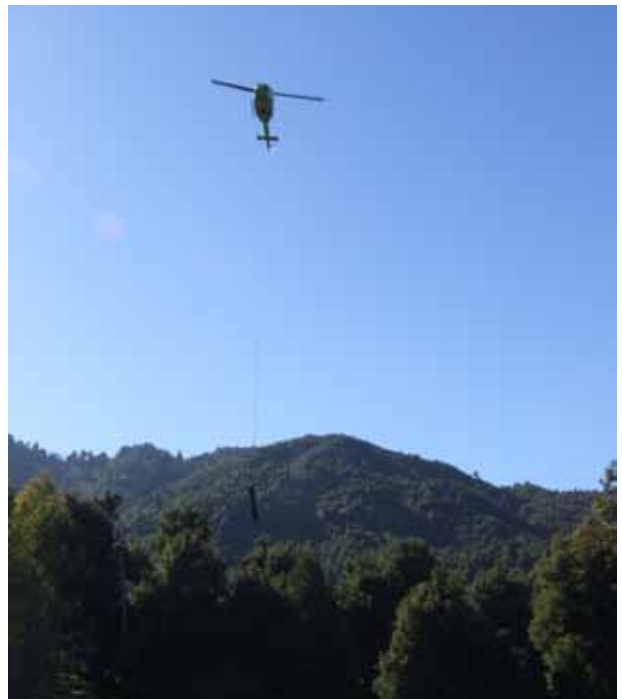
The Iroquois helicopter is about to land a tawa log from the Otekura bush at the Tahora milling site.
