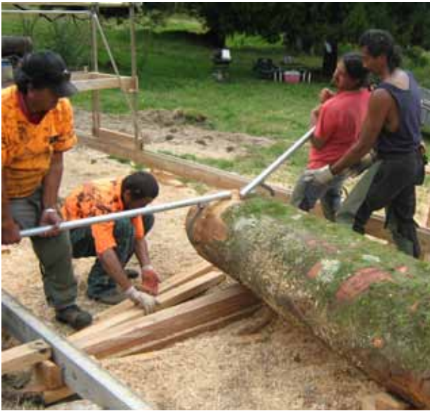
Some good logs came out for this trial, giving the team some work with cant hooks to get the logs into position for the mill. On the right, Elvis Miki helps miller Rob Mansell while Raymond Te Kurapa positions a platform for the log. On the left, Pat Mansell heaves on the other cant hook!
