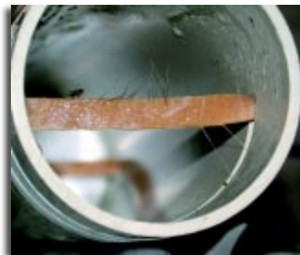
■ A stoat-hair-collecting tube, showing sticky rubber band to catch the hair.
