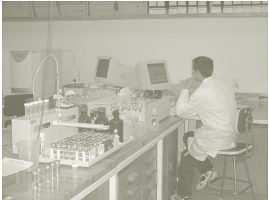
The Lachat FIA analysing leachate samples
