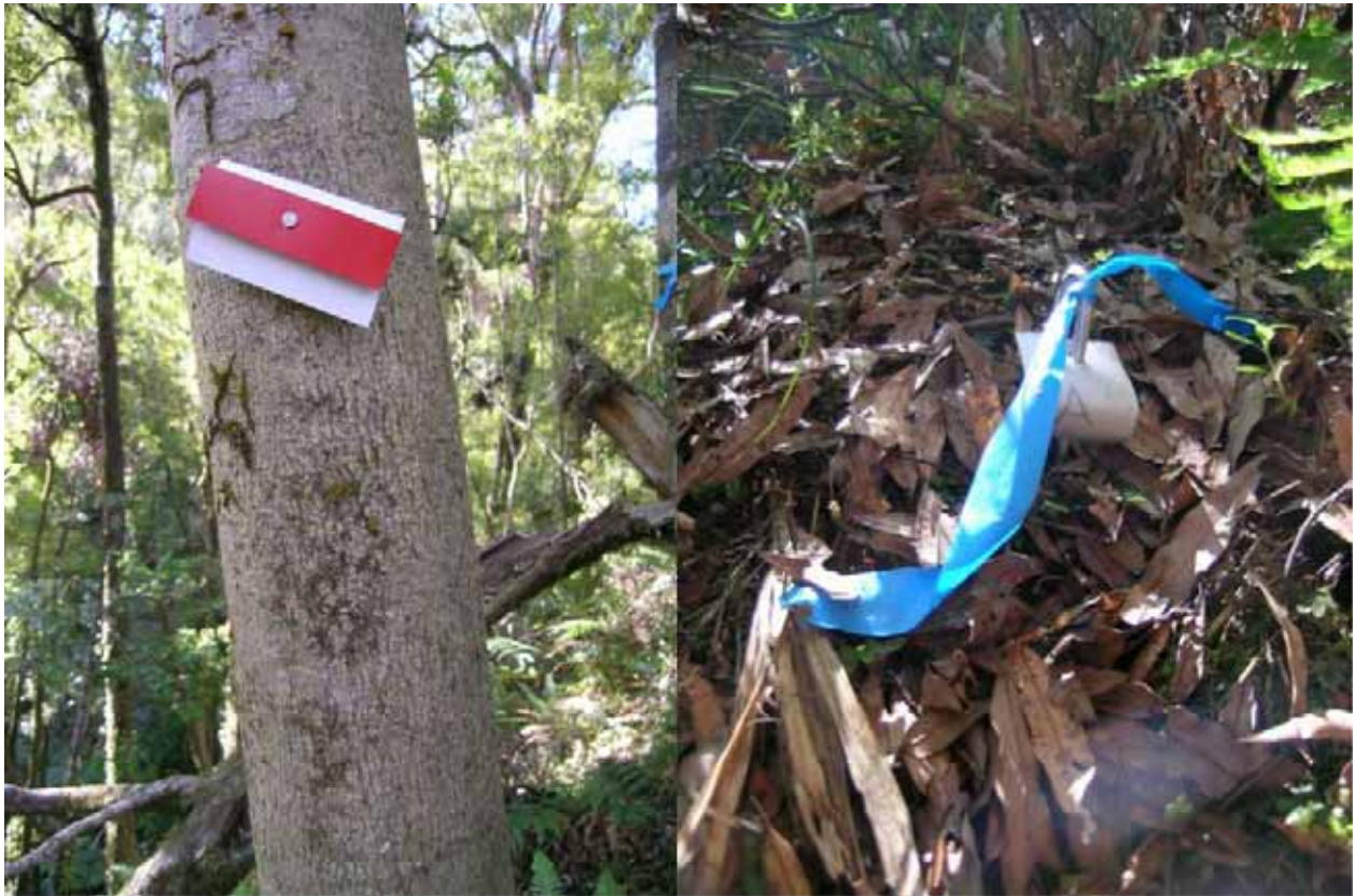
The four corners of each plot are marked with red and white Permatag while the corners are marked on the ground using metal pegs, Permatag and flagging tape.
