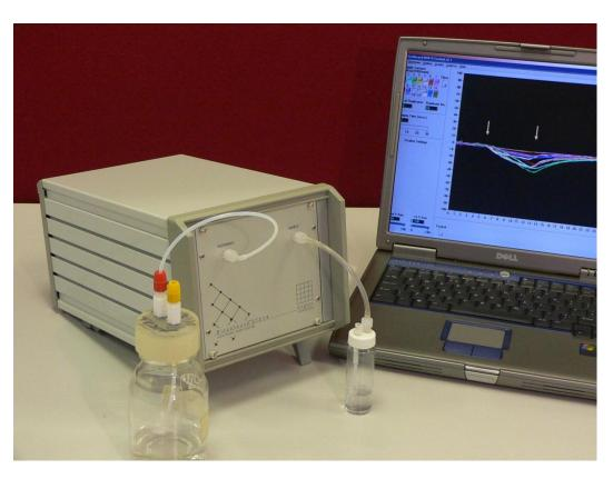
Flow injection system (pulse or sniff of volatiles to give transient response)
