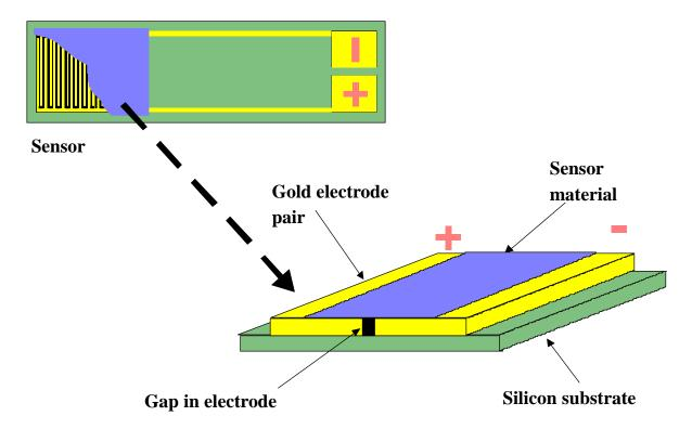
The resistance of the polymer material deposited on the electrode changes when volatile chemicals interact with the surface.
