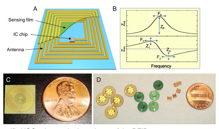
Specific VOCs change the impedance of the RFID sensor antenna
