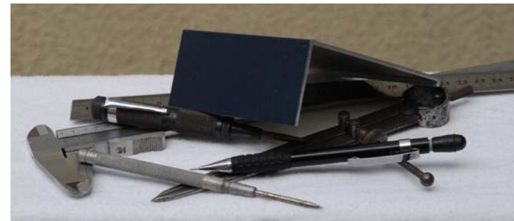
Above L to R: callipers, ruler, scribe, centre punch, dividers and pencil with the powder-coated aluminium resting on top of the tools.
