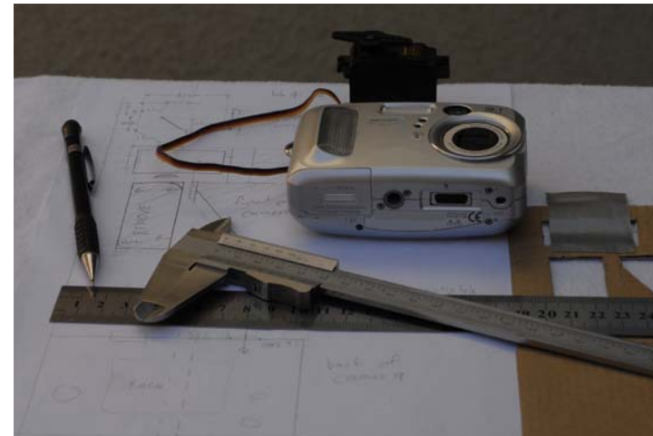
Above L to R: pencil, ruler, callipers, digital camera, servomotor and cardboard template all sitting on top of a working drawing of the adaptor plate.
