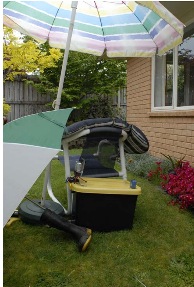
A prototype time lapse camera controller set up on ice plant flowers that open in direct sunlight. The time clock adds information on time to each image. An umbrella makes an effective temporary shelter for protecting equipment from rain and the heat of the sun during a photo shoot in marginal weather conditions. The gumboot helps anchor an umbrella when it is windy.
