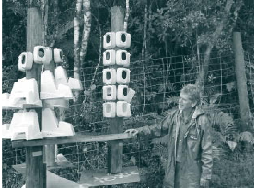
Fig. 1. Gel baits and pellet baits in bait stations mounted on “possum-proof” poles in a bait-weathering enclosure.
