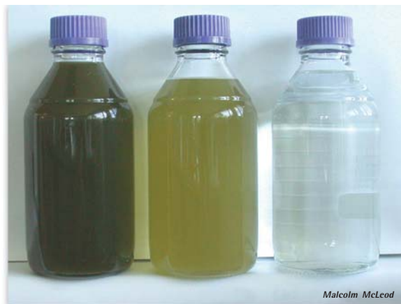
■ An informative comparison: Left: Raw dairy shed effluent. Centre: Leachate collected from 25 millimetres of effluent and 10 millimetres of rainfall applied to a clay soil. Right: The same leachate from a pumice soil.
