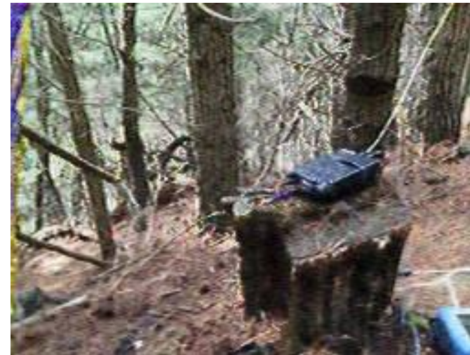
SSTV transmission over 500m distance in forested terrain
