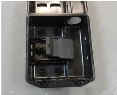
Figure 4. Unset T-Rex rat trap in an open Sidekick bait station. Left: Trap placed fully back in the trap recess so that rats had access to the front edge of the trap, as used for test 3. Right: Trap placed forward in the trap recess so that the leading edge of the trap was flush with the wall of the bait station. This set was used for test 4.
