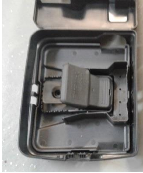
Figure 2. A set un-baited T-Rex rat trap inside an open Ambush bait station. The entrance holes in the bait station base are on the right and are offset from where the trap is positioned so rats approach the trap from around a corner. The Ambush bait station was used for tests 1 and 2.
