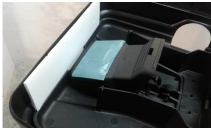
Figure 3. Unset T-Rex rat trap in an open Ambush bait station showing the added corflute barrier. When the bait station was closed, the barrier was held securely by the station roof in a vertical orientation.
