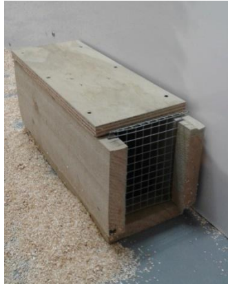
Figure 5. The Predator Free NZ wooden trap tunnel used for tests 5 and 6. A 50 × 50 mm entrance hole was cut in the mesh at the far end of the tunnel (not visible) and the mesh at the closed end of the tunnel was removable to allow access to the trap. The T-Rex trap was set 2 cm into the tunnel from the closed end. Two tacks were nailed into the trap tunnel floor in front of the trap to prevent it being pulled forward, or pushed too close to the entrance hole in the front mesh.
