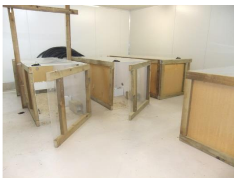
Figure 1. The four arenas used for trap testing. Rats were provided with a nest box, had free access to water, and were fed with standard rodent pellets (ProLab RHM 1800 LabDiet, PMI Nutrition International, MO, USA). Arenas are shown with Predator Free NZ wooden trap tunnels in place.
